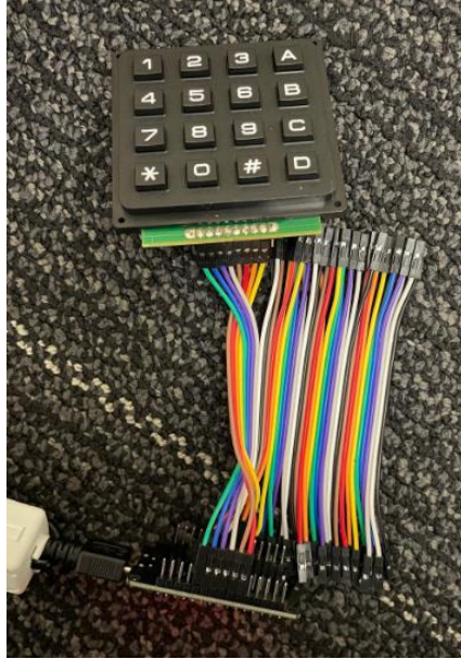
Figure 46: Keypad Connected for Testing
