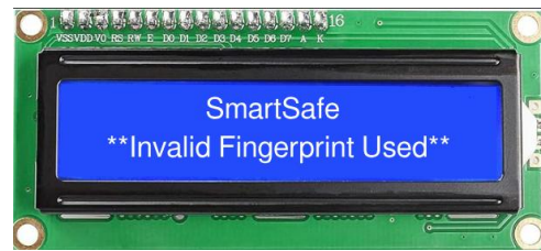
Figure 38: Display Invalid Prototype
